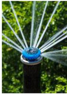
MP Rotators and Toro Precisions to the new RainBird RVAN nozzles, there is a high efficiency nozzle for every situation. An important thing to remember is that each brand has a different flow and precipitation rate and will need different runtimes to apply 1.5" of water a week to turf grass in the summer, never mix any nozzle types on the same zone. Hunter MP's ( 0.41 in/hr or (0.81 in/hr -800 series), Toro Precision (1.0 in/hr), RainBird RVAN (0.61 in/hr).
