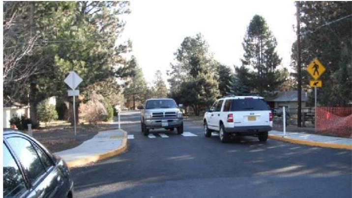
Figure 16 Raised Pedestrian Crossing/Speed Table
