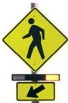
Figure 8 RRFB with LED Stutter Flash
